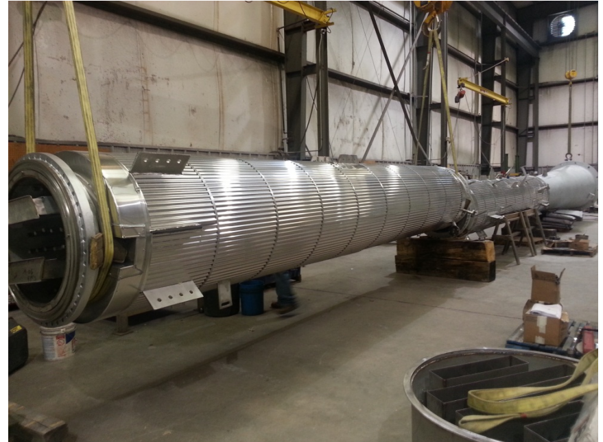
Stripper section in fabrication and assembly
