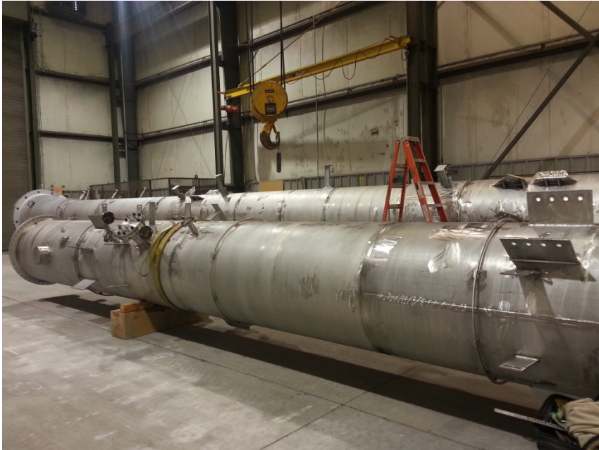
Absorber section in fabrication and assembly
