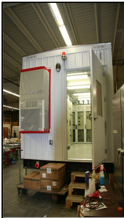
Analyzer and controls container
